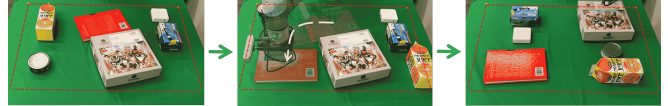
Fig. 1: A motivating example in developing RVG. In object rearrangement, high-quality paths often need to be planned to translate and rotate objects in a 2D workspace, e.g., a tabletop. Images are reproduced from [1].
